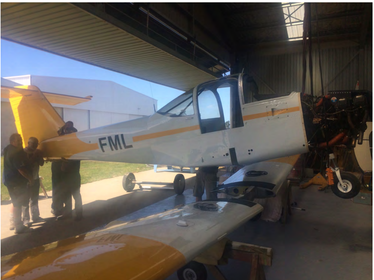
6. Jay and his team remounting the fuselage onto the wings.
